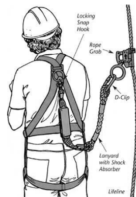
Figure 2. Components of a Personal Fall Arrest System
