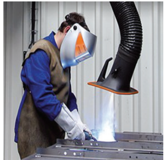
Figure 1: Welder using extraction ventilation.
