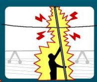
Never raise irrigation pipes without checking for safe distances from power lines.
