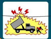
Don't approach a vehicle that is in contact with a power line.
