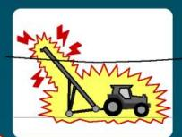
Always lower a portable grain auger before moving it.
